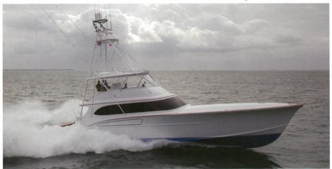
Delivered to South Florida, the *FULL TIME* is the latest offering from Paul Mann. When tested for its final performance numbers, the boat (with tower attached and with 16 crew aboard) went 45 kt (52 MPH) WOT. Even at 1250 RPMs tests showed over 18 kt. She's equipped with state-of-the-art 16-cylinder Tier 3 MTU Series 2000 M96 engines. These brawny built for long-distance power plants not only generate up to 2600 HP per engine, but also have a power-to-weight ra-
