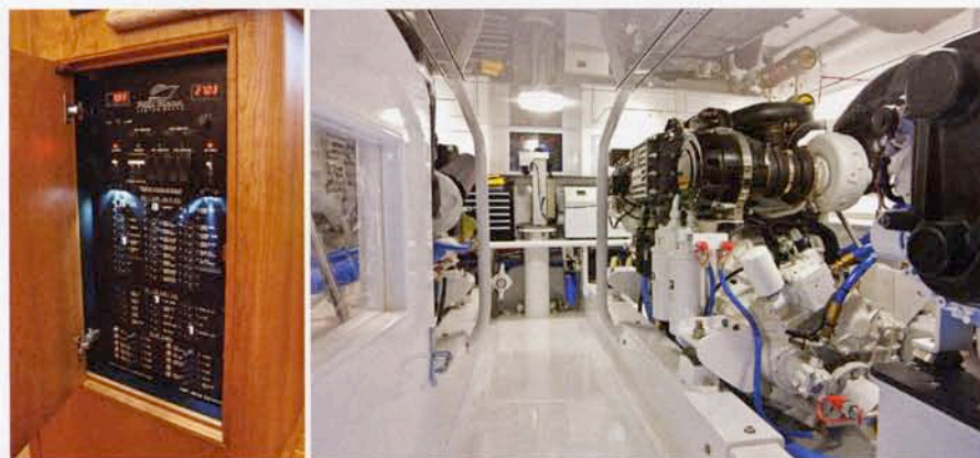
Alina's spacious engine room holds twin C18s and has enough room to satisfy Paul Mann's "two hands on anything you need to fix" credo.
